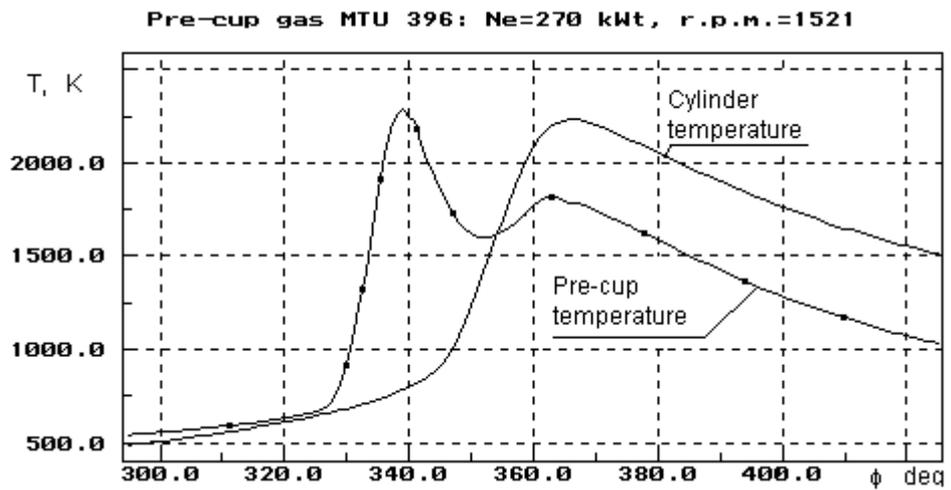
Fig 4. The in-cylinder average temperature and pre-chamber temperature.
