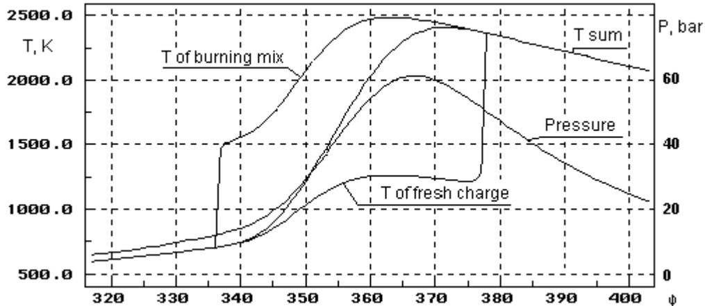
Fig 1. Curves of pressure and temperatures in the zones during combustion in SI petrol engine.
