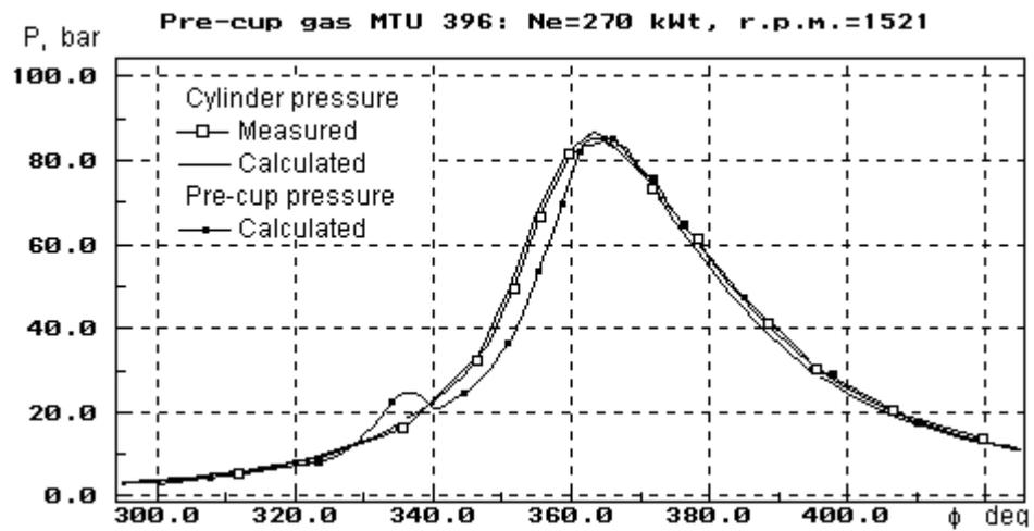
Fig 3. Pressure in the cylinder and in pre-chamber.
