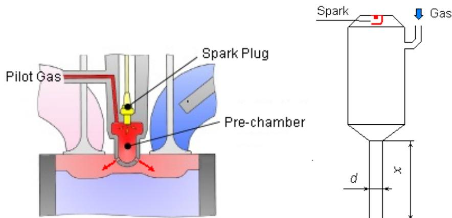
Fig 2. Scheme of pre-chamber.
