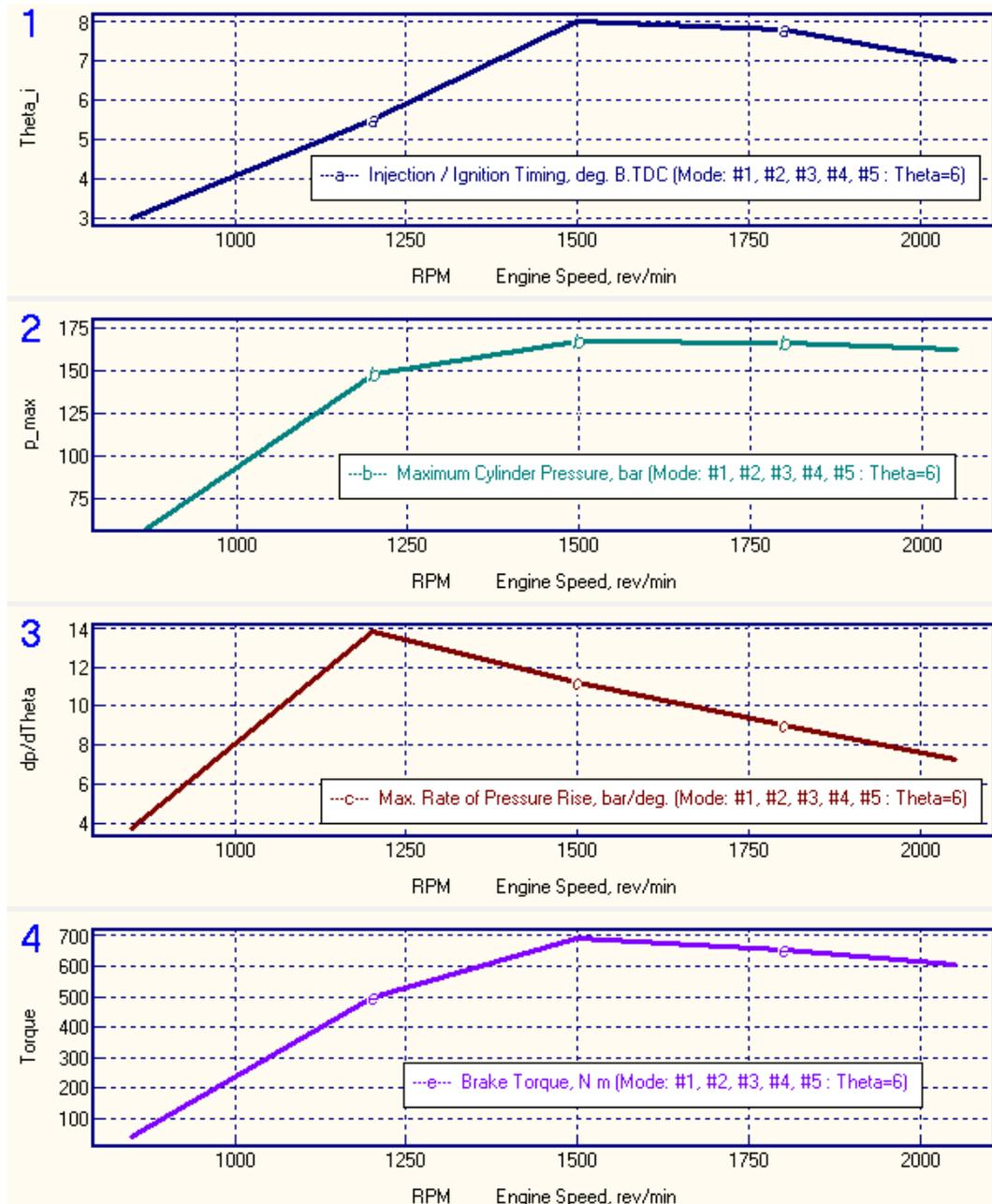
Figure 16. The change of the following engine parameters vs. RPM: (a) Fuel injection timing  $\Theta_{i,i}$  [deg. BTDC], (b) Maximum cylinder pressure  $p_{max}$  [bar], (c) The rate of pressure rise  $dp/d\theta$  [bar/degree], (d) Torque  $Torque$  [Nm].
