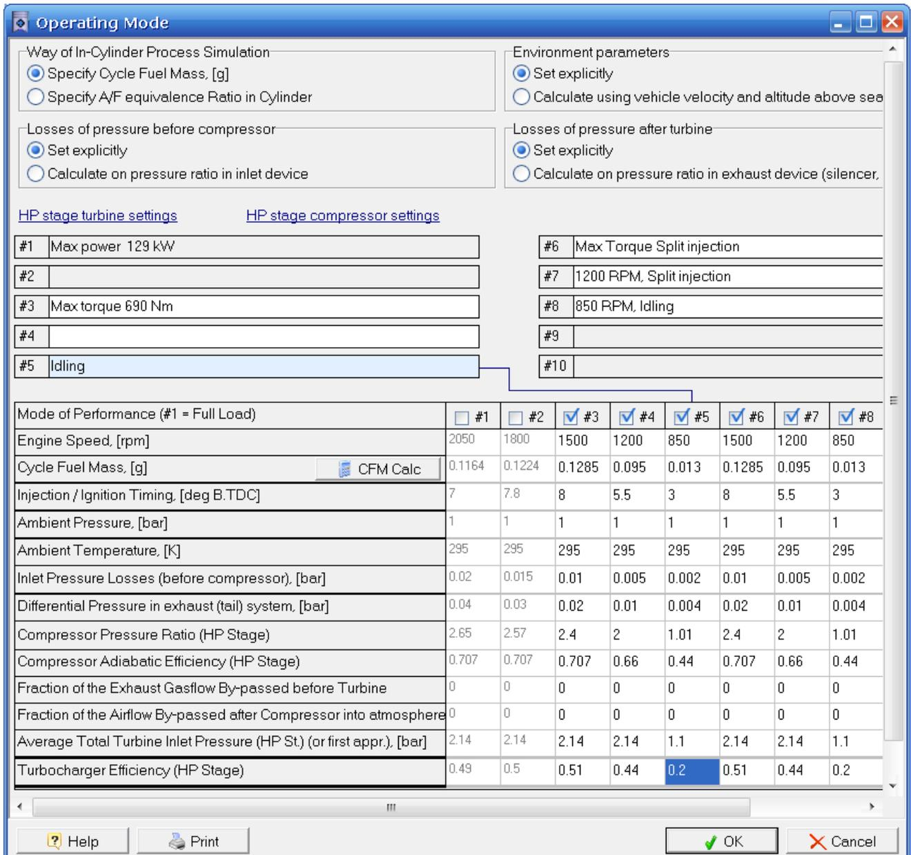
Figure 17. Selection of additional regimes No. 6, and 7 for the engine output characteristics.
