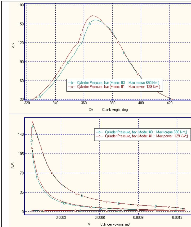
Figure 13. Comparison of in-cylinder pressure diagrams [bar] as a function of RPM and cylinder volume.
