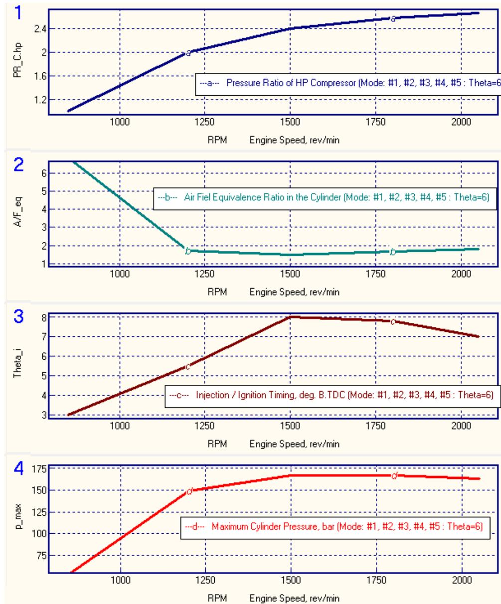
Figure 12. The change of engine parameters vs. RPM: (1) Compressor pressure ratio,  $PR_c$ , (2) Air fuel equivalence ratio,  $A/F_{eq}$ , (3) Fuel injection timing,  $\Theta_i$  [deg. BTDC], (4) Maximum cylinder pressure,  $p_{max}$  [bar]
