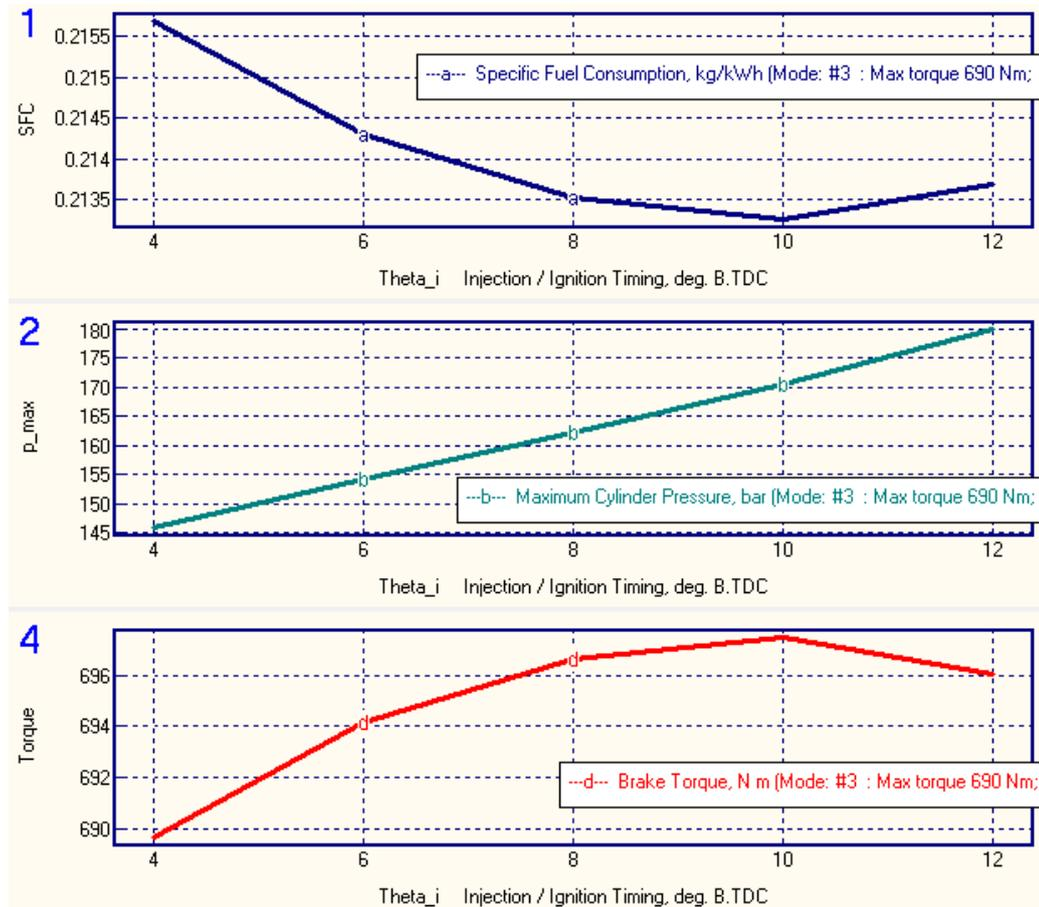
Figure 6. Dependence of the specific fuel consumption SFC [kg/kWh], the maximum cylinder pressure  $p_{max}$  [bar] and torque on fuel injection timing  $\Theta_{i}$  at maximum torque regime.
