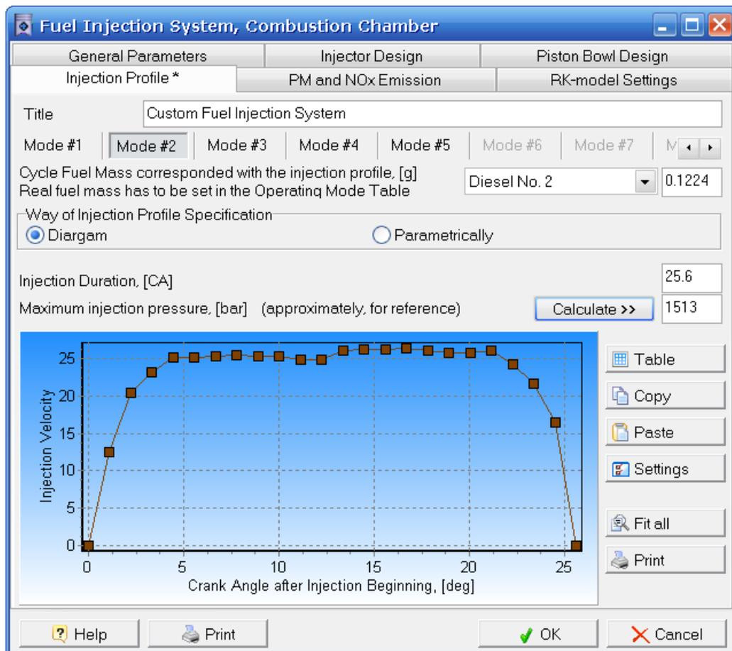
Figure 9. Injection characteristics for intermediate higher power regime (1800 RPM).
